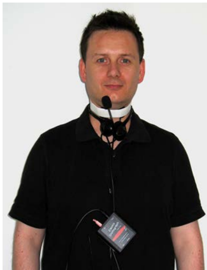
Figure 4: The author of the present work. Experimental setup with the portable VoceVista electro-glottograph and the connected headset microphone.
