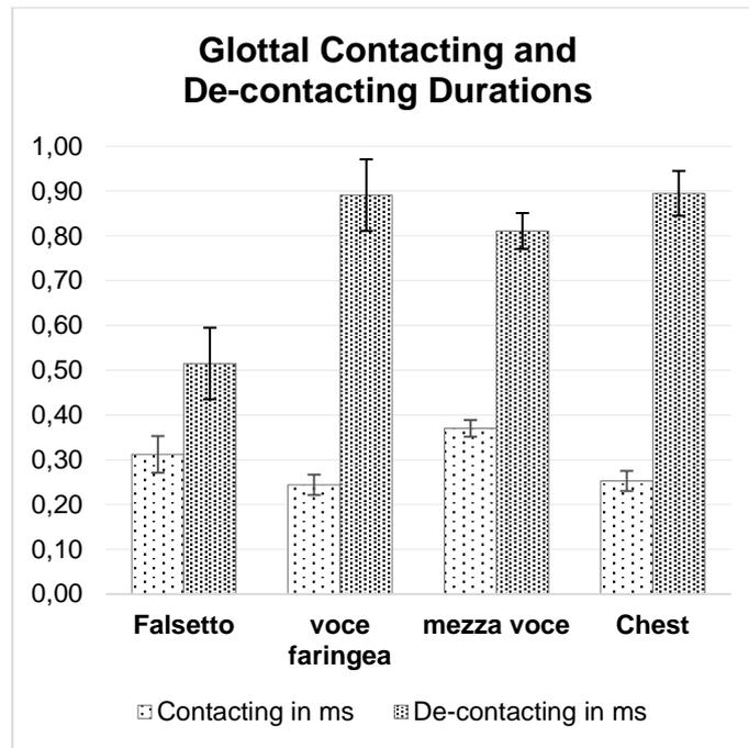
**FIGURE 4.** Comparison of the glottal contacting and de-contacting durations in ms in falsetto, *voce faringea*, *mezza voce* (B4) and chest register of sustained tones sung on the vowel /a/ on C5 measured over a period of 500 ms by the Eggworks software.
