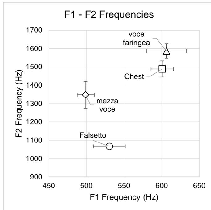
**FIGURE 7.** Average frequencies and standard deviations of the first and second formants of the vowel /a/ sung on C5 in falsetto, *voce faringea*, *mezza voce* (B4) and chest register estimated by means of the Burg algorithm, embedded in the Praat software.
